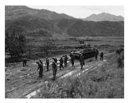
Engineers probing for hidden mines ahead of a slowly moving M4A3E8 medium tank near Ch'orwon
